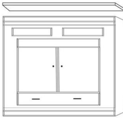
B TOP Finished Top Piece that sits on top to hide unfinished wood
