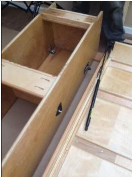
Set the tray on the floor face down and attach the piston to the tray adjustable brackets with the smaller shaft end attached as soon. (Note: set the tray at least 4 feet from the wall the bed will be mounted to. (shown left) This is so there is room to get behind the unit to attach the pistons in step 6)
